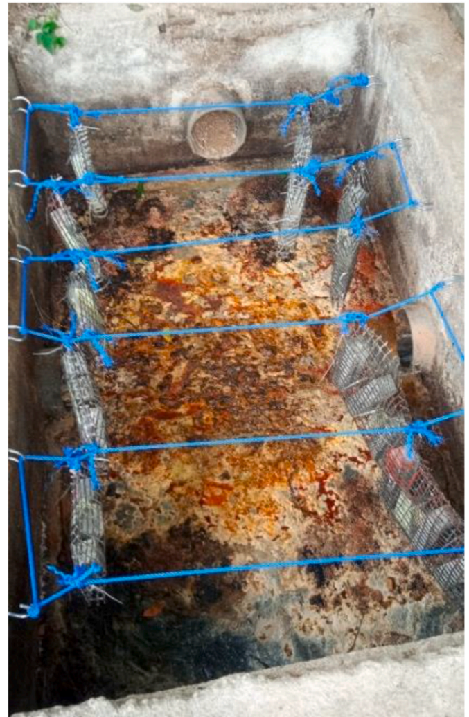
Fig. 5. Suspension of prismatic paste specimens above water level at Location B.
